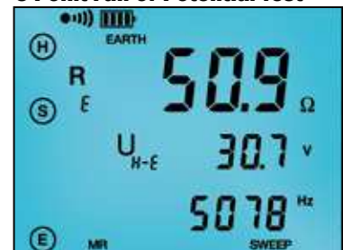
The 3-Point Fall-of-Potential test displays test lead connection, grounding rod resistance and test electrode resistances.
