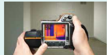
Infrared cameras quickly locate moisture related problems
