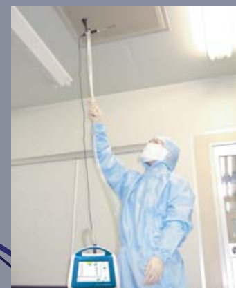
Climomaster™ probe for environmental measurements
