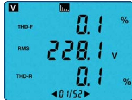
Displays THD, % and value for each harmonic to the 50 th with one screen for each harmonic.
