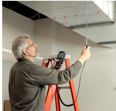
Duct traverse with Micromanometer and pitot tube
