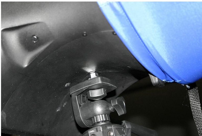
Figure 27: Mount Hood Base to Telescopic Stand
