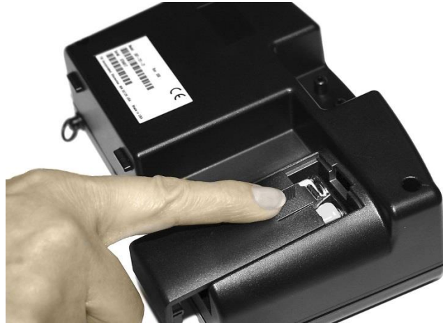
Figure 5: Battery Cover Removal
