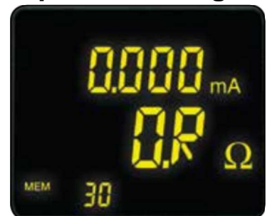
Indicates that the impedance is greater than 1500Ω
